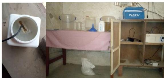
Figure 2 - Photo of an electro-chlorinator device and a production room.
